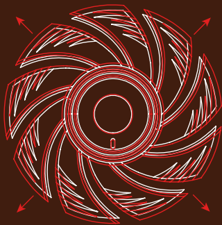
Impeller creep due to centrifugal forces
