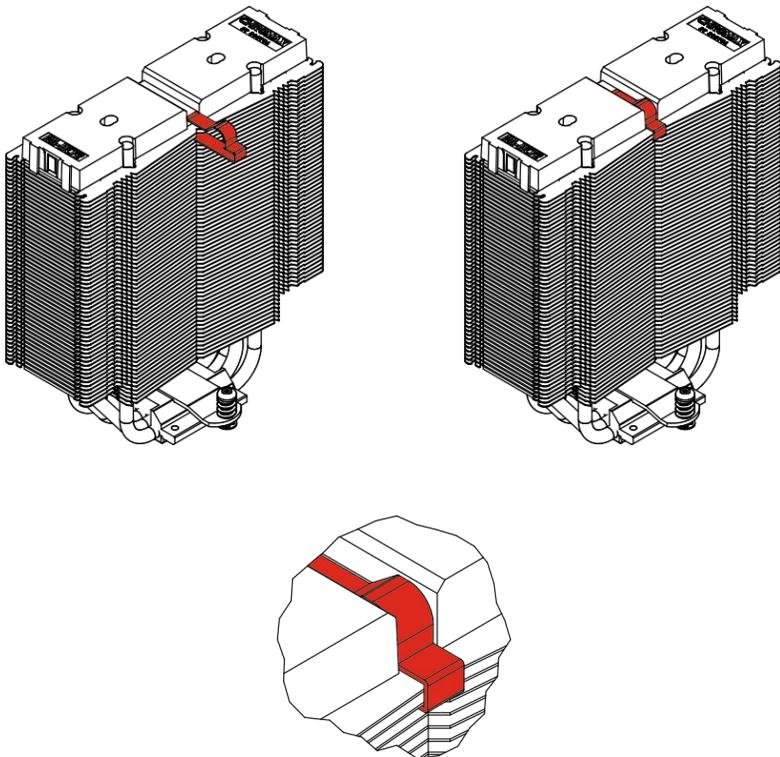
Note that the steel clip must go underneath the second fin from the top.
