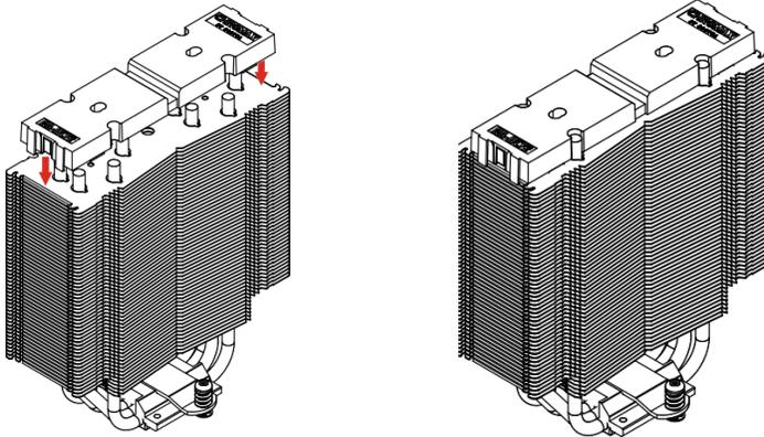
**2** Attach the fixture to the heatsink using the steel clip.
