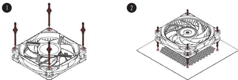
If the long ends of the mounts are in the way, you can use scissors to cut them after installation. Note that this will then make them difficult to reinstall in the future.
