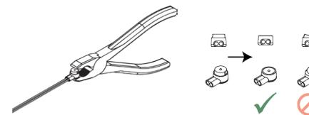
After you've fixed the original fan's cable to the OmniJoin adaptor using the Skotchlok™ connectors, simply connect the NF-A12x25 5V to the adaptor in order to use it in your device.
