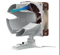
The air that comes out of an axial fan has a high amount of rotational energy, which results in a helix-shaped flow path. The AAS recovers this rotational energy and uses it to accelerate the airflow. With the inside shape of the AAS funnel carefully fine-tuned to the helix structure produced by the NF-A12x25 fan, it achieves an extremely high rate of energy recovery.
