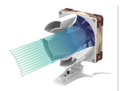
Following the principle of mass continuity, a fluid's speed increases when it's forced through a reduced cross-sectional area, so when the air is driven through the progressively narrowing AAS funnel, air speed increases continuously until it reaches maximum velocity at the outlet.
