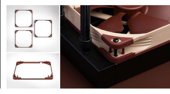
The NA-SAVG2 is a set of three NA-AVG2 anti-vibration gaskets for using compatible Noctua 140x25mm fans on water cooling radiators or other applications that benefit from a tighter seal with the fan. Made from extra soft yet highly tear-proof silicone rubber, the NA-AVG2 help to damp minute vibrations and to reduce air loss between the fan and the radiator. As such, they are an ideal accessory for performance enthusiasts who want to squeeze out those extra few percent of cooling efficiency.
