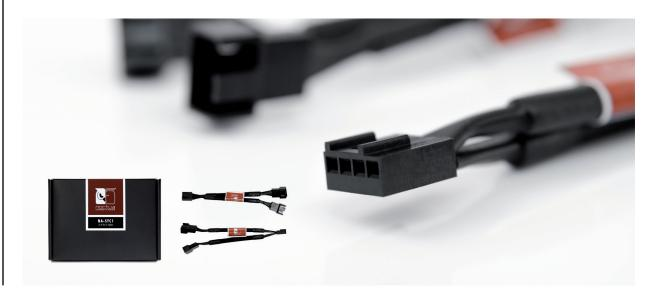
The NA-SYC1 is a fan accessory set consisting of two fully sleeved NA-YC1 Y-Cables for 4-pin PWM fans. The NA-YC1 Y-Cables make it possible to run two 4-pin PWM fans on a single fan header and to let the mainboard control the speed of both fans simultaneously. Multiple NA-YC1 can be daisy-chained to control more than two PWM fans via one header.
