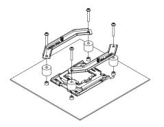
Please note that this NM-AM5/4-MP78 kit is compatible with heatsinks with 78mm mounting pitch only. For heatsinks with 83mm mounting pitch, the NM-AM5/4-MP83 kit must be used instead.
