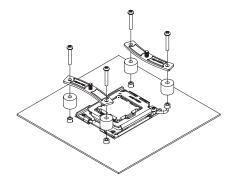
Please note that this NM-AM5/4-MP83 kit is compatible with heatsinks with 83mm mounting pitch only.
