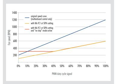
"No stop" mode can be used in order to avoid motherboard fan errors that can occur below certain speed levels or if the fan stops. To exit "no stop" mode, press the "no stop" mode push button 3 again, so that the green "no stop" mode status LED 4 goes off.
