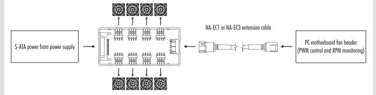
If both its S-ATA and 4-pin input ports are connected, the NA-FH1 will automatically draw power via S-ATA and use the 4-pin port for PWM control and RPM monitoring only. This way, it is possible to control fans with high power consumption safely without risking damage to the motherboard.
