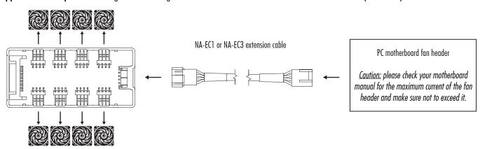
Application example 2: Controlling high-current PC PWM fans safely via a motherboard fan header using S-ATA power (54W max.)
