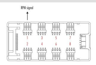
The NA-FH1 transmits the RPM speed signal of the fan connected to the first port to the motherboard for speed monitoring. For additional watchdog functionality, all ports feature status LEDs that light up if an RPM signal is being received and go off if the fan stops or fails.
