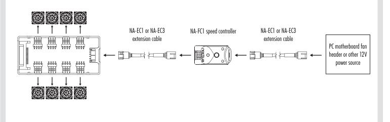
Application example 4: Powering high-current 12V PWM fans through the S-ATA connector and controlling them using NA-FC1 (54W max.)
