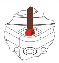
If the long ends of the mounts are in the way, you can use scissors to cut them after installation. Note that this will then make them difficult to reinstall in the future.
