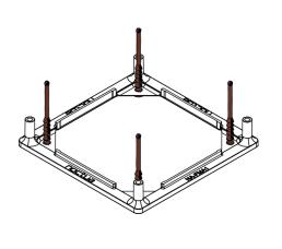
Then put on the 120x25mm fan so that the tips of the anti-vibration mounts stick through the fan's mounting holes. Pull on the tips to fix the fan until pawl number 5 is all the way through.
