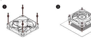
If the long ends of the mounts are in the way, you can use scissors to cut them after installation.
