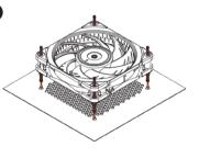
If the long ends of the mounts are in the way, you can use scissors to cut them after installation. Note that this will then make them difficult to reinstall in the future.
