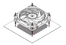
If the long ends of the mounts are in the way, you can use scissors to cut them after installation. Note that this will then make them difficult to reinstall in the future.
