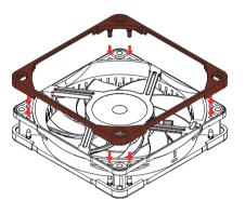
The NA-AVG1 gasket can also be used for other applications that benefit from a tighter seal with the fan.
