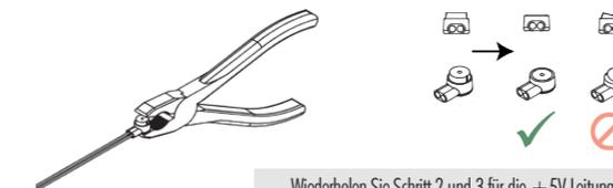
After you've fixed the original fan's cable to the OmniJoin adaptor using the cable connectors, simply connect the NF-A20 5V to the adaptor in order to use it in your device.
