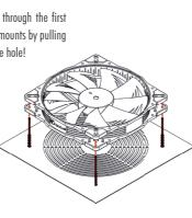
If the long ends of the mounts are in the way, you can use scissors to cut them after installation
