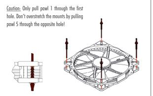
Then pull the C side through the mounting holes of the case.
