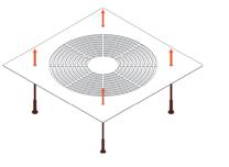
Then pull the tip through the fan's mounting holes until the pawl 1 is all the way through the hole.
