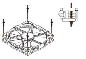
Then pull the C side through the mounting holes of the case.
