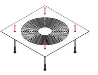
Then pull the tip through the fan's mounting holes until the pawl 1 is all the way through the hole.
