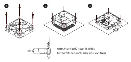
Then pull the C side through the mounting holes of the case. If the long ends of the mounts are in the way, you can use scissors to cut them after installation.
