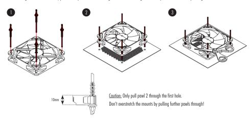
Then pull the C side through the mounting holes of the case. If the long ends of the mounts are in the way, you can use scissors to cut them after installation.
