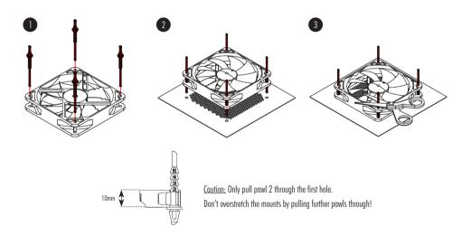
Then pull the C side through the mounting holes of the case. If the long ends of the mounts are in the way, you can use scissors to cut them after installation.
