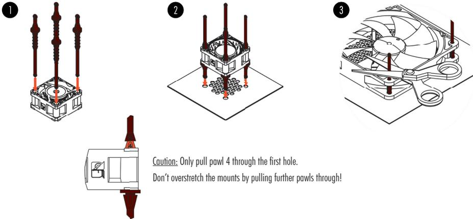
Then pull the C side through the mounting holes of the case. If the long ends of the mounts are in the way, you can use scissors to cut them after installation. Note that this will then make them difficult to reinstall in the future.
