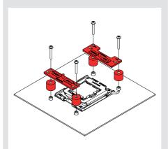
On AM5 and Ryzen 5000/3000 series AM4 CPUs, choose the -7mm offset hole position to ensure optimal contact quality and performance.
