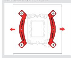
Fix the mounting bars using the four NM-STS1 thumb screws.
