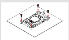
On AM4, the stock backplate will become loose when unscrewing the retention module, so hold it in place for the next step. If you have lost your stock AM4 backplate, please contact us at <a href="mailto:support@noctua.at">support@noctua.at</a>. On AM5, the stock backplate is screw-fixed to the socket, so should simply remain in place.
