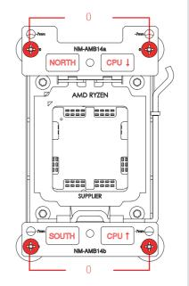
Caution: Make sure that the "CPU  $\rightarrow$ " markings point towards the CPU and that the NM-AMB14a bar with the "NORTH" marking is installed on the north (top) side of the socket and the NM-AMB14b bar with the "SOUTH" marking is installed on the south (bottom) side of the socket, as shown above.
