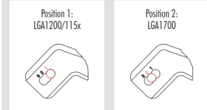
**Caution:** Make sure to use the correct hole position on both ends of the NM-IMB3 mounting bars so that they will not be misaligned.
