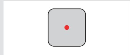
**Caution:** Applying too much thermal paste will lower heat conductivity and cooling performance!
