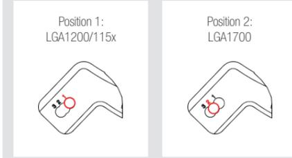
**Caution:** Make sure to use the correct hole position on both ends of the NM-IMB2 mounting bars so that they will not be misaligned.
