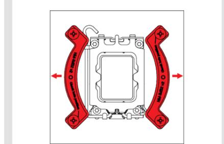
Fix the mounting bars using the four NM-ITS1 thumb screws.
