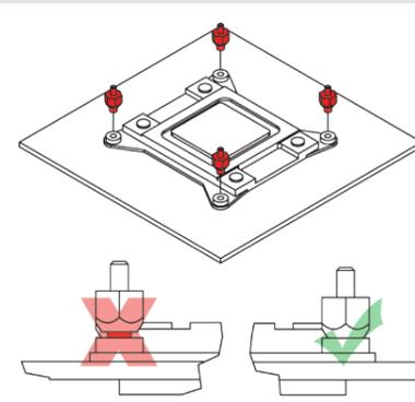
Then put the NM-IMB2 mounting bars onto the bolts.
