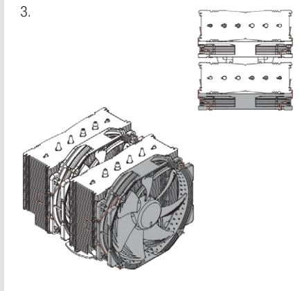
Use the heatsink with the centre fan only in order to guarantee best compatibility with tall RAM modules. Add the second fan to the front fin stack for further improved cooling performance.
