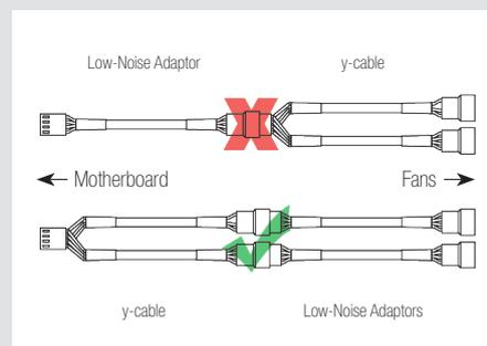
**Caution:** When using the L.N.A.s, check the temperature of your CPU using appropriate software (e.g. the respective applications of your motherboard manufacturer), in order to evade automatic throttling of the CPU due to the increased temperature. If the cooling performance is insufficient, please increase case ventilation or remove the L.N.A.s.
