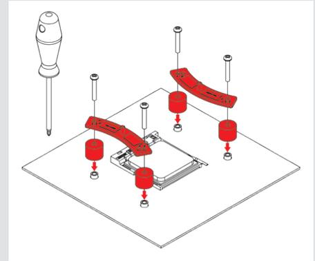
Make sure that the curved sides of the mounting bars are pointing inwards.
