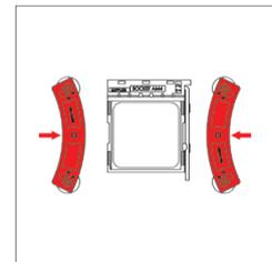
**Caution:** Gently tighten the screws until they stop, but do not use excessive force (max. torque 0.6 Nm).
