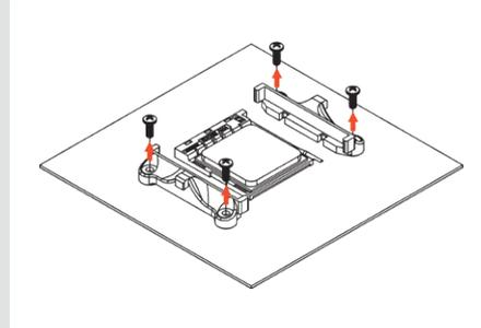
If your motherboard does not come with a pre-installed CPU cooler retention module, the AMD stock backplate should be included with the motherboard accessories. Please put the backplate on the rear side of the motherboard so that the screw threads of the backplate stick through the mounting holes of the motherboard as shown below. If your motherboard does not include a stock backplate, please contact Noctua customer support at [support@noctua.at](mailto:support@noctua.at).
