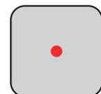
**Caution:** Applying too much thermal paste will lower heat conductivity and cooling performance!
