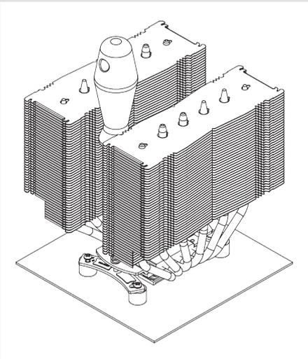
**Caution:** Gently tighten the screws until they stop, but do not use excessive force (max. torque 0.6 Nm).
