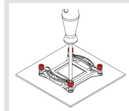
**Caution:** Gently tighten the screws until they stop, but do not use excessive force (max. torque 0.6 Nm).
