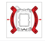
Fix the mounting bars using the four NM-ITS1 thumb screws.
