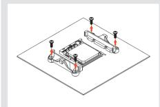
If your motherboard does not come with a pre-installed CPU cooler retention module, the AMD stock backplate should be included with the motherboard accessories. Please put the backplate on the rear side of the motherboard so that the screw threads of the backplate stick through the mounting holes of the motherboard as shown below. If your motherboard does not include a stock backplate, please contact Noctua customer support at support@noctua.at.
