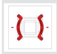
Fix the mounting bars using the four NM-ITS1 thumb screws.
