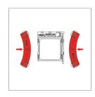
Caution: Gently tighten the screws until they stop, but do not use excessive force (max. torque 0.6 Nm).
