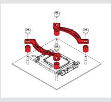
Caution: Choose the alignment of the mounting bars according to the desired final orientation of the cooler:
