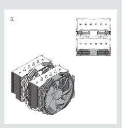
Use the heatsink with the centre fan only in order to guarantee best compatibility with tall RAM modules. Add the second fan to the front fin stack for further improved cooling performance.
