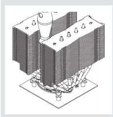
Caution: Gently tighten the screws until they stop, but do not use excessive force (max. torque 0.6 Nm).
