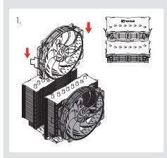
For increased RAM clearance, the front fan can also be moved upwards. Please note, however, that this will increase the total cooler height beyond 168mm:
