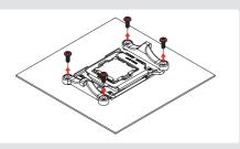
On AM4, the stock backplate will become loose when unscrewing the retention module, so hold it in place for the next step. If you have lost your stock AM4 backplate, please contact us at support@noctua.at. On AM5, the stock backplate is screw-fixed to the socket, so should simply remain in place.
