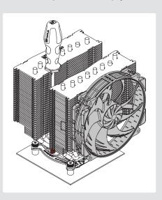
Caution: Gently tighten the screws until they stop, but do not use excessive force (max. torque 0.6 Nm).
