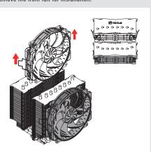
Then put the heatsink onto the CPU and screw it to the screw threads of the mounting bars. Perform 2-3 turns on each screw, then repeat until both are fully tightened.
