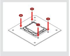
Put the ILM back into place and secure it using the 4 original screws. Gently tighten the screws until they stop, but do not use excessive force (max. torque 0.6 Nm).
