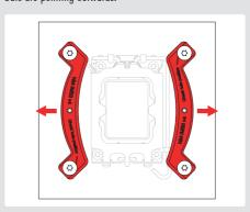
Fix the mounting bars using the four NM-STS1-TX thumb
