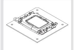
If the screws do not catch the threads easily, apply slight pressure onto the screws and first turn them counterclockwise until you hear a clicking sound as the threads fall into place, then start turning clockwise. If necessary, reach behind the motherboard and apply counterpressure to the backplate to help the screws catch the thread. If the screws still don't catch the thread, please contact us at support@ noctua.at so that we can supply you with longer screws.
