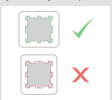
Apply 5 dots; 4 small dots with  $\sim$ 2mm diameter near the corners plus 1 dot with 3-4mm diameter in the centre:
