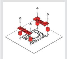
On AM5 and Ryzen 5000/3000 series AM4 CPUs, choose the -7mm offset hole position to ensure optimal contact quality and performance.
