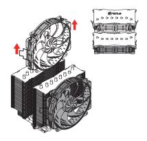
Then put the heatsink onto the CPU and screw it to the screw threads of the mounting bars. Perform 2-3 turns on each screw, then repeat until both are fully tightened.
