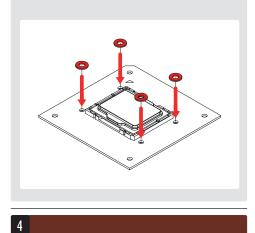
Put the ILM back into place and fix it using the original 4 screws. Gently tighten the screws until they stop, but do not use excessive force (max. torque 0.6 Nm).
