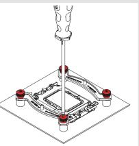
: Gently tighten the screws until they stop, but do excessive force (max. torque 0.6 Nm).
