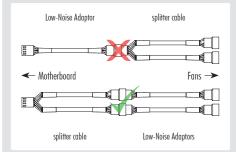
Caution: When using the L.N.A.s, check the temperature of your CPU using appropriate software (e.g. the respective applications of your motherboard manufacturer), in order to evade automatic throttling of the CPU due to the increased temperature.
