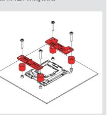
On AM5 and Ryzen 5000/3000 series AM4 CPUs, choose the -7mm offset hole position to ensure optimal contact quality and performance.
