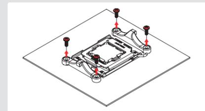
On AM4, the stock backplate will become loose when unscrewing the retention module, so hold it in place for the next step. If you have lost your stock AM4 backplate, please contact us at [support@noctua.at](mailto:support@noctua.at). On AM5, the stock backplate is screw-fixed to the socket, so should simply remain in place.
