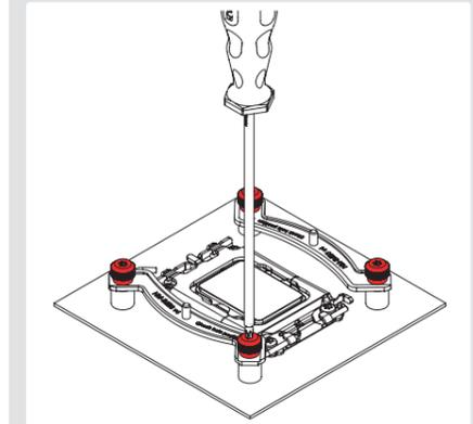
**Caution:** Gently tighten the screws until they stop, but do not use excessive force (max. torque 0.6 Nm).
