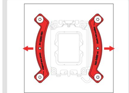
Fix the mounting bars using the four NM-ST51-TX thumb screws.
