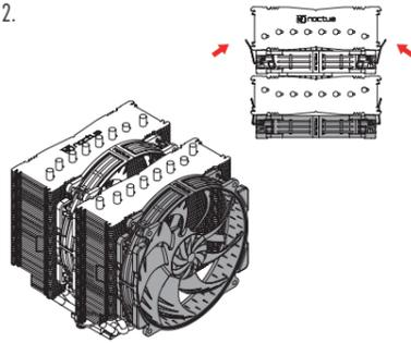
For increased RAM clearance, the front fan can also be moved upwards. Please note, however, that this will increase the total cooler height beyond 168mm:
