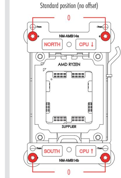
**Caution:** Make sure that the "CPU →" markings point towards the CPU and that the NM-AMB14a bar with the "NORTH" marking is installed on the north (top) side of the socket and the NM-AMB14b bar with the "SOUTH" marking is installed on the south (bottom) side of the socket, as shown above.
