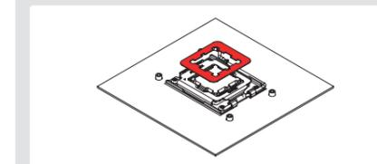
Make sure that the inner opening of the guard is correctly aligned with the outer edges of the heat-spreader:
