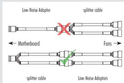
**Caution:** When using the L.N.A.s, check the temperature of your CPU using appropriate software (e.g. the respective applications of your motherboard manufacturer), in order to evade automatic throttling of the CPU due to the increased temperature.
