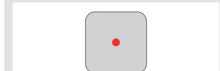
**Caution:** Applying too much thermal paste will lower heat conductivity and cooling performance!
