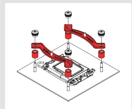
**Caution:** Choose the alignment of the mounting bars according to the desired final orientation of the cooler.
