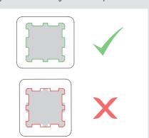
Apply 5 dots; 4 small dots with  $\sim$ 2mm diameter near the corners plus 1 dot with 3-4mm diameter in the centre:
