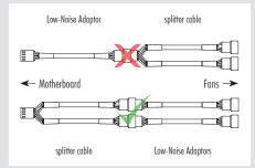
Caution: When using the L.N.A.s, check the temperature of your CPU using appropriate software (e.g. the respective applications of your motherboard manufacturer), in order to evade automatic throttling of the CPU due to the increased
