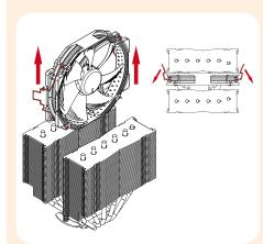
Then put the heatsink onto the CPU and screw it to the screw threads of the mounting bars.
