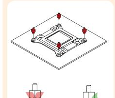
Then put the NM-IMB2 mounting-bars onto the bolts.
