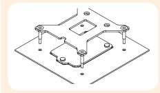
Caution: The supplied backplate will install over the mainboard's stock backplate, so the mainboard's stock backplate must not be
