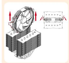
Then put the heatsink onto the CPU and screw it to the screw threads of the mounting bars.
