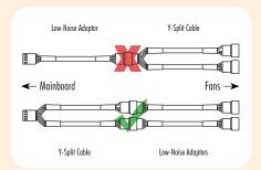
Caution: When using the L.N.A.s, check the temperature of your CPU using appropriate software (e.g. the respective applications of your mainboard manufacturer), in order to evade automatic throttling of the CPU due to the increased temperature. If the cooling performance is insufficient, please increase case ventilation or remove the L.N.A.s.
