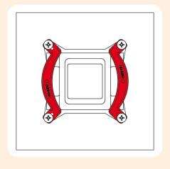
Fix the mounting bars using the 4 thumb screws.
