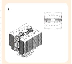
Connect the fan to the mainboard's CPU fan header. Depending on your CPU and the temperature inside the case, you may interconnect the supplied NA-RC7 Low-Noise Adapter (L.N.A.) in order to further reduce the fan's operating noise.
