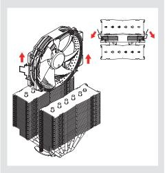
Then put the heatsink onto the CPU and screw it to the screw threads of the mounting bars.
