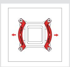
Fix the mounting bars using the four NM-ITS1s thumb
