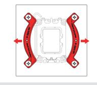
Fix the mounting bars using the four NM-ITS1s thumb screws.
