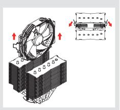
Then put the heatsink onto the CPU and screw it to the screw threads of the mounting bars. Perform 2-3 turns on each screw, then repeat until both are fully tightened.
