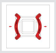
Fix the mounting bars using the four NM-ITS1 thumb
