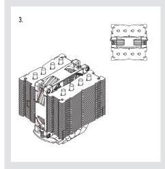
Connect the fan to the motherboard's CPU fan header.
