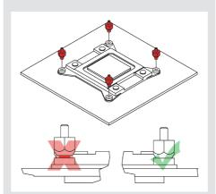
Then put the NM-IMB2 mounting bars onto the bolts.
