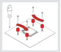
Make sure that the curved sides of the mounting bars are pointing inwards.
