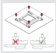
Then put the NM-IMB3 mounting bars onto the bolts.
