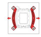
Fix the mounting bars using the four NM-ITS1 thumb
