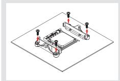
If your motherboard does not come with a pre-installed CPU cooler retention module, the AMD stock backplate should be included with the motherboard accessories.
