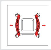
Fix the mounting bars using the four NM-ITS1 thumb screws.
