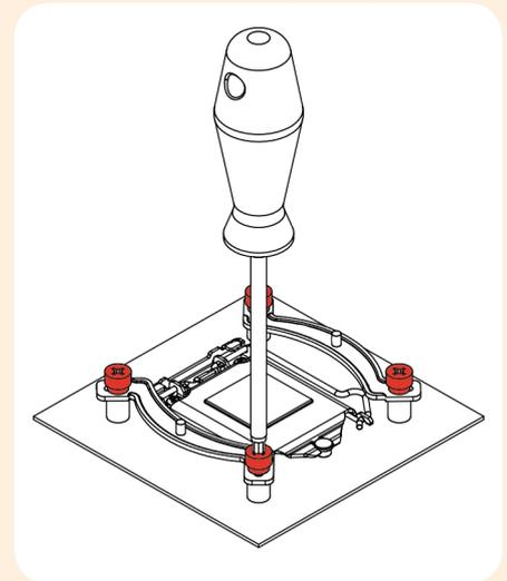
**Caution:** Gently tighten the screws until they stop, but don't use excessive force (max. torque 0.6 Nm).
