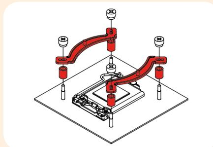
**Caution:** Choose the alignment of the mounting bars according to the desired final orientation of the cooler:
