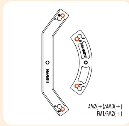
Choose either the short NM-AMB10 or the long NM-AMB11 mounting bars according to the desired final orientation of the cooler.
