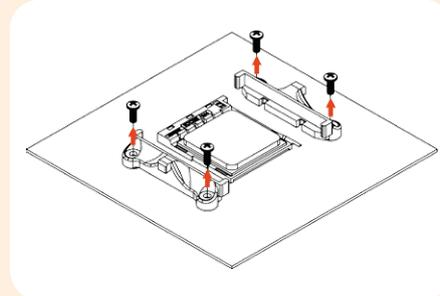
If your motherboard does not come with a pre-installed CPU retention module, the AMD stock backplate should be included with the motherboard accessories. Please put the backplate on the rear side of the motherboard so that the screw-threads of the backplate stick through the mounting holes of the motherboard as shown below. If your motherboard does not include a stock backplate, please contact Noctua customer support at [support@noctua.at](mailto:support@noctua.at).
