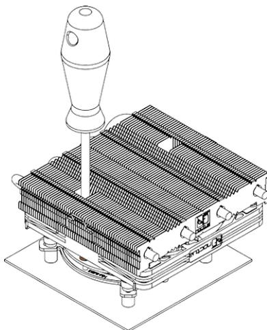
**Caution:** Gently tighten the screws until they stop, but don't use excessive force (max. torque 0.6 Nm).
