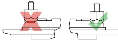
Then put the NM-IMB3 mounting-bars onto the bolts.
