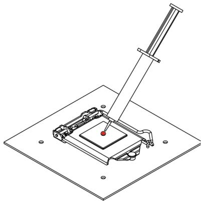
**Caution:** Applying too much thermal paste will lower heat conductivity and cooling performance!
