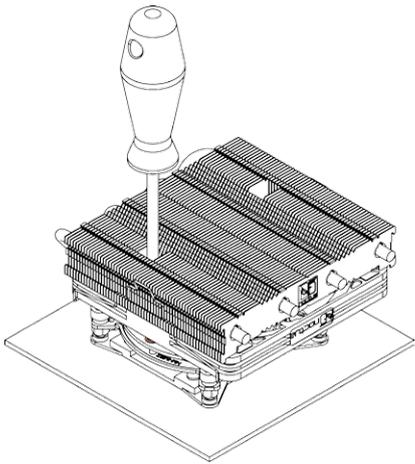
**Caution:** Gently tighten the screws until they stop, but don't use excessive force (max. torque 0.6 Nm).
