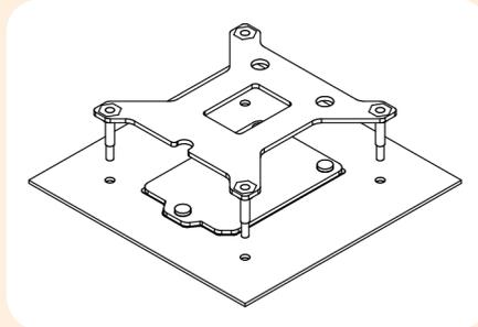
**Caution:** The supplied backplate will install over the motherboard's stock backplate, so the motherboard's stock backplate must not be taken off.
