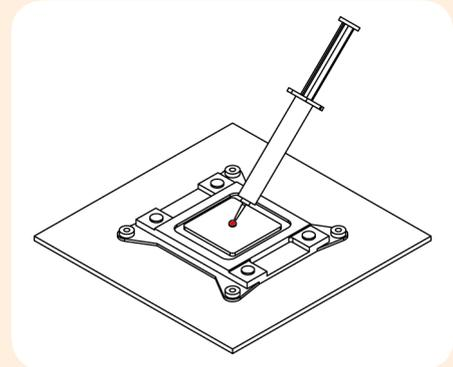
**Caution:** Applying too much thermal paste will lower the heat conductivity and cooling performance!
