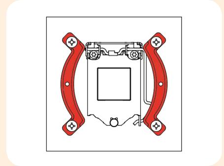
Fix the mounting bars using the 4 thumb screws.
