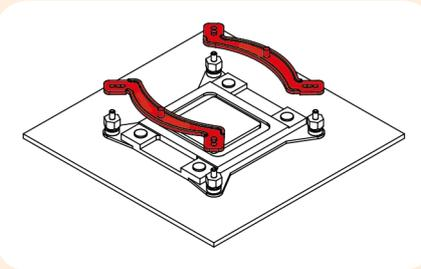
**Caution:** Choose the alignment of the mounting bars according to the desired final orientation of the cooler:
