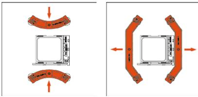
**Caution:** Gently tighten the screws until they stop, but don't use excessive force (max. torque 0.6 Nm).
