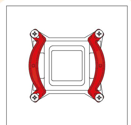
Fix the mounting bars using the 4 thumb screws.
