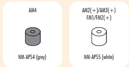
Use the grey NM-APS4 spacers for AM4 and the white NM-APS5 spacers for AM2(+)/AM3(+)/FM1/FM2(+).
