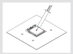
Caution: Applying too much thermal paste will lower heat conductivity and cooling performance!
