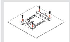
If your motherboard does not come with a pre-installed CPU cooler retention module and backplate, please proceed with
