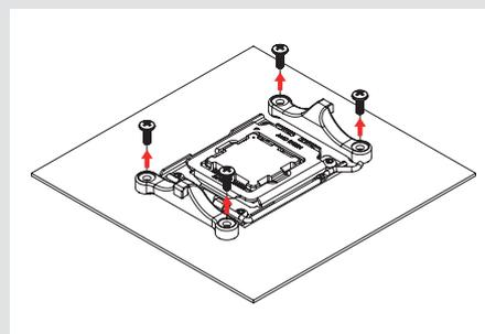
Do not unscrew the backplate from the socket; it must be kept in place.
