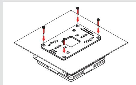
Begin fixing the screws by hand and then use the supplied mounting tool to tighten. Perform 3 turns on each screw, then repeat until all are fully tightened.
