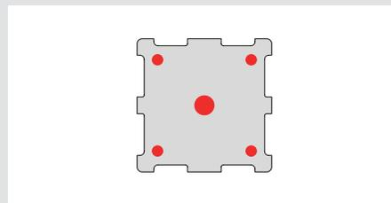
**Caution:** Applying too much thermal paste will lower heat conductivity and cooling performance!
