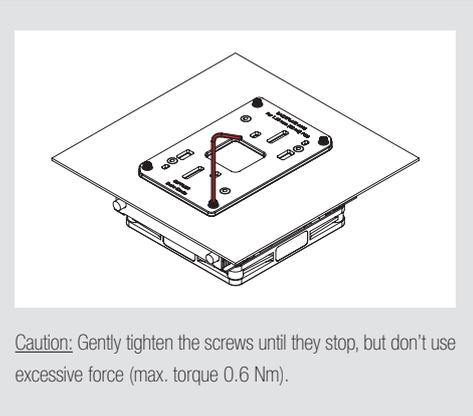
**Caution:** Gently tighten the screws until they stop, but don't use excessive force (max. torque 0.6 Nm).
