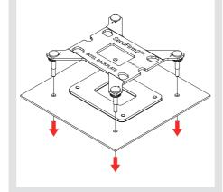
Caution: The supplied backplate will install over the motherboard's stock backplate, so the motherboard's stock backplate must not be taken off.
