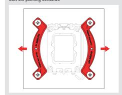
Fix the mounting bars using the four NM-ITS1 thumb
