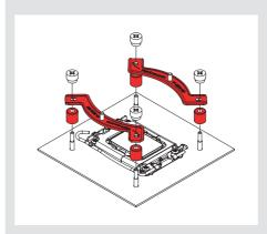
Caution: Choose the alignment of the mounting bars according to the desired final orientation of the cooler.
