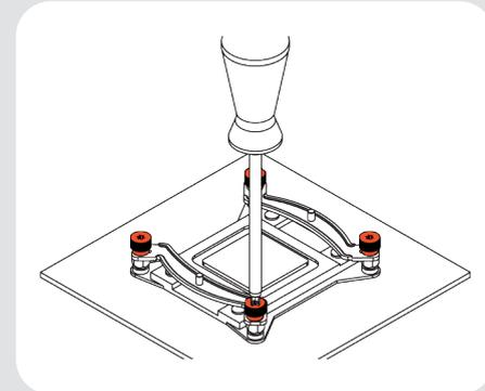
**Caution:** Gently tighten the thumb screws until they stop, but do not use excessive force (max. torque 0.6 Nm).
