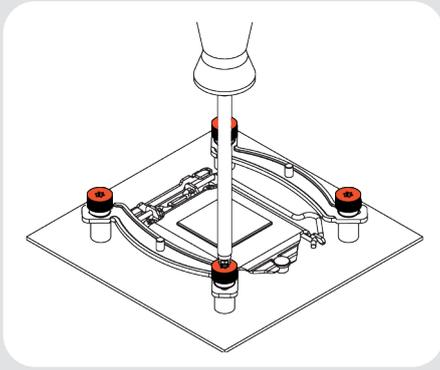
**Caution:** Gently tighten the thumb screws until they stop, but do not use excessive force (max. torque 0.6 Nm).
