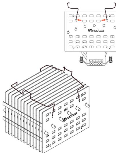
Place the fan on the heatsink and pull the clips over the fan to hold it in place.
