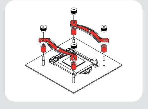
**Caution:** Choose the alignment of the mounting bars according to the desired final orientation of the cooler.
