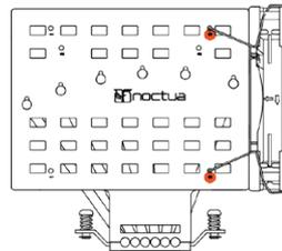
Then insert the tips of the fan clips into the correct hole set.
