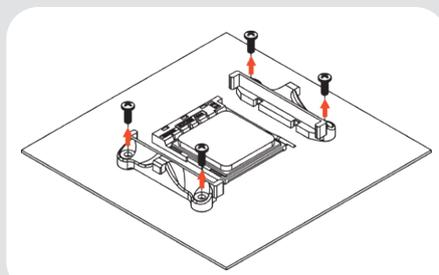
If your motherboard does not come with a pre-installed CPU cooler retention module, the AMD stock backplate should be included with the motherboard accessories. Please put the backplate on the rear side of the motherboard so that the screw threads of the backplate stick through the mounting holes of the motherboard as shown below. If your motherboard does not include a stock backplate, please contact Noctua customer support at [support@noctua.at](mailto:support@noctua.at).
