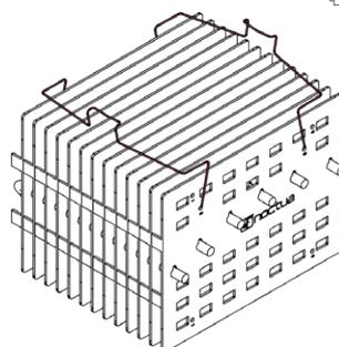
Place the fan on the heatsink and pull the clips over the fan to hold it in place.
