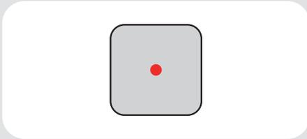
**Caution:** Applying too much thermal paste will lower heat conductivity and cooling performance!
