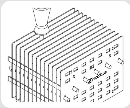
**Caution:** Gently tighten the screws until they stop, but do not use excessive force (max. torque 0.6 Nm).
