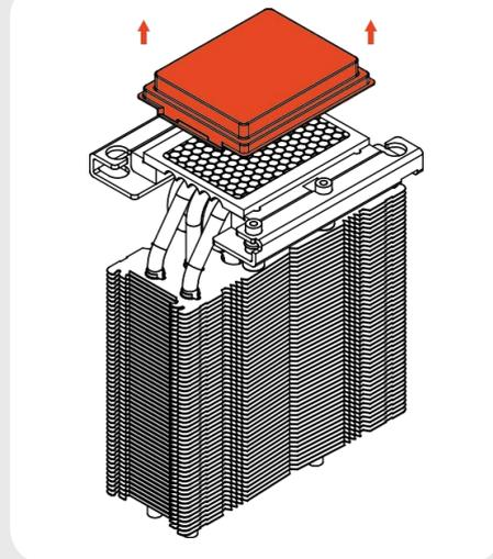
Turn the heatsink upside down so that the base is facing upwards. Carefully put it down onto the tips of the heatpipes and secure it with your hand so that it cannot tilt and that the fins cannot get bent. Remove the plastic protection cover from the base of the heatsink and be careful not to damage the layer of pre-applied thermal compound.
