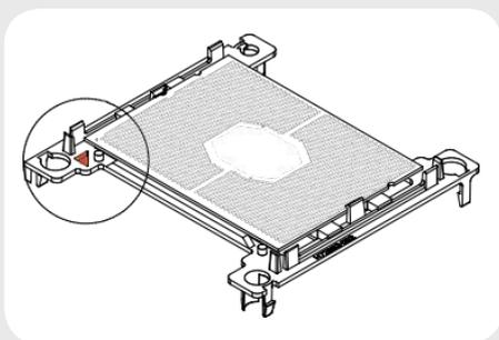
**Caution:** Some LGA3647 CPUs have a so called OmniPath fabric connector. If your CPU is of this type, you need a different processor clip. Please contact [support@noctua.at](mailto:support@noctua.at) if you have a CPU with OmniPath fabric connector.
