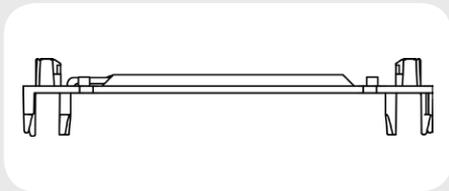
Orient the CPU so that the heatspreader is facing downwards and the golden contacts are facing upwards. Be careful not to touch the contacts. Then put the CPU into the clip, aligning the CPU's pin 1 (golden triangle indicator) with the triangle pin 1 indicator of the clip. Snap the CPU into the clip. Note that you may need to flex the clip a bit for it to latch onto the CPU. Verify that the clip is fully attached to the CPU before proceeding.
