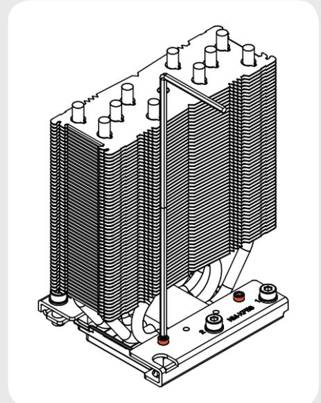
**Caution:** Gently tighten the screws until they stop, but don't use excessive force (max. torque 0.6 Nm).
