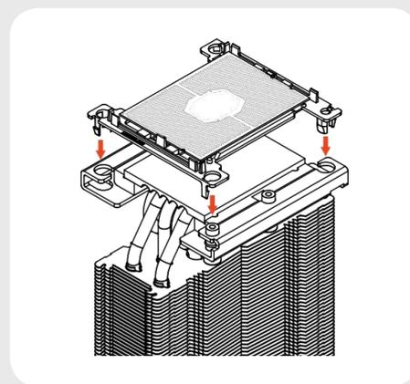
Verify that all the latches have snapped to the mounting brackets and that the CPU and clip are fully attached to the heatsink.
