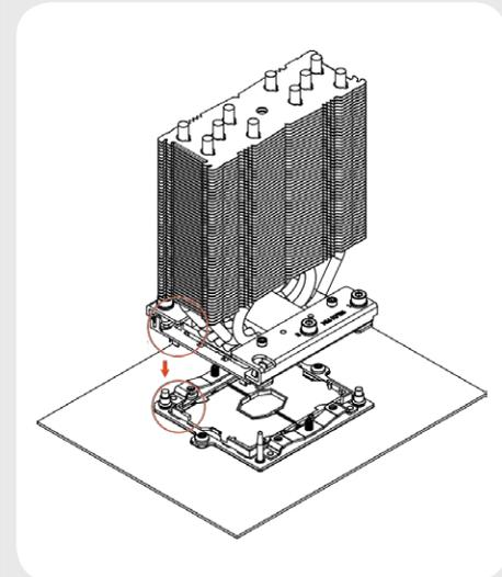
Start fastening the heatsink to the socket by tightening the outer screws (number 1), starting with the screw at pin 1.
