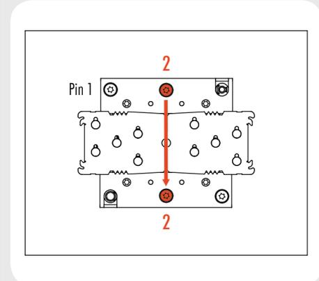
**Caution:** Gently tighten the screws until they stop, but don't use excessive force (max. torque 0.8 Nm).
