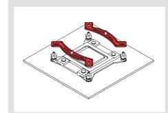
Caution: Choose the alignment of the mounting bars according to the desired final orientation of the cooler:
