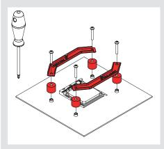
Make sure that the curved sides of the mounting bars are pointing outwards.
