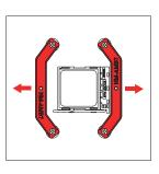
Caution: Gently tighten the screws until they stop, but do not use excessive force (max. torque 0.6 Nm).
