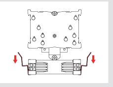
Then put the heatsink onto the CPU and screw it to the screw threads of the mounting bars.
