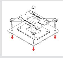
Caution: The supplied backplate will install over the motherboard's stock backplate, so the motherboard's stock backplate must not be taken off.
