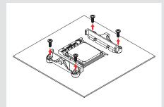
If your motherboard does not come with a pre-installed CPU cooler retention module, the AMD stock backplate should be included with the motherboard accessories. Please put the backplate on the rear side of the motherboard so that the screw threads of the backplate stick through the mounting holes of the motherboard as shown below. If your motherboard does not include a stock backplate, please contact our Noctua service team at support@noctua.at.
