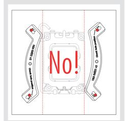
Put the plastic spacers onto the bolts of the backplate, then add the mounting bars.
