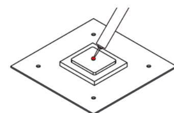
**Caution:** Applying too much thermal paste will lower the heat conductivity and cooling performance!
