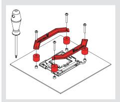
Make sure that the curved sides of the mounting bars are pointing outwards.
