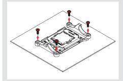
The SecuFirm2 $^{\text{TM}}$  mounting system will install directly to the stock backplate, so please keep it in place.
