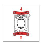
$\underline{\text{Caution:}}$  Gently tighten the screws until they stop, but do not use excessive force (max. torque 0.6 Nm).
