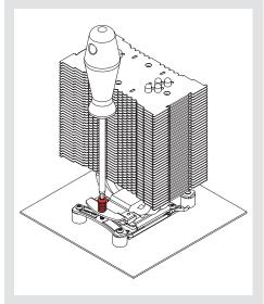
$\underline{\text{Caution:}}$  Gently tighten the screws until they stop, but do not use excessive force (max. torque 0.6 Nm).
