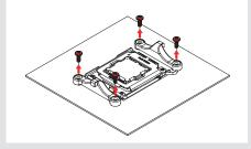
The SecuFirm2  $^{\text{TM}}$  mounting system will install directly to the stock backplate, so please keep it in place.
