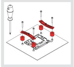
Make sure that the curved sides of the mounting bars are pointing inwards.
