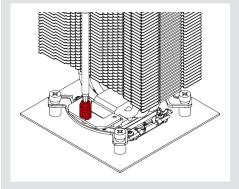
$\underline{\text{Caution:}}$  Gently tighten the screws until they stop, but do not use excessive force (max. torque 0.6 Nm).
