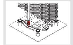
Caution: Gently tighten the screws until they stop, but do not use excessive force (max. torque 0.6 Nm).
