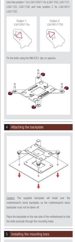
Please first choose the correct set of plastic spacers and the correct set of holes on the mounting bars according to whether you are using an LGA1200/LGA115x (LGA1150. LGA1151, LGA1155, LGA1156) or an LGA1851/LGA1700 socket motherboard.
