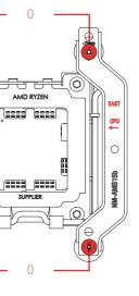
marking is installed on the west (left) side of the socket and the NM-AMB15b bar with the "EAST" marking is installed on the
