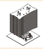
When employing the 90° fastening brackets, please use the supplied mounting-tool to tighten the springscrews.
