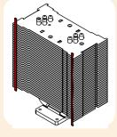
Then attach the fan to the heatsink using the 2 steel clips, placing it so that it blows onto the heatsink (You can optionally use the second pair of clips to install a second fan).
