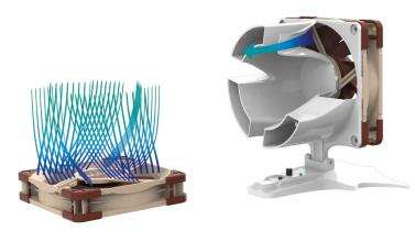
The air that comes out of an axial fan has a high amount of rotational energy, which results in a helix-shaped flow path. The AAS recovers this rotational energy and uses it to accelerate the airflow. With the inside shape of the AAS funnel carefully fine-tuned to the helix structure produced by the NF-A12x25 fan, it achieves an extremely high rate of energy recovery.
